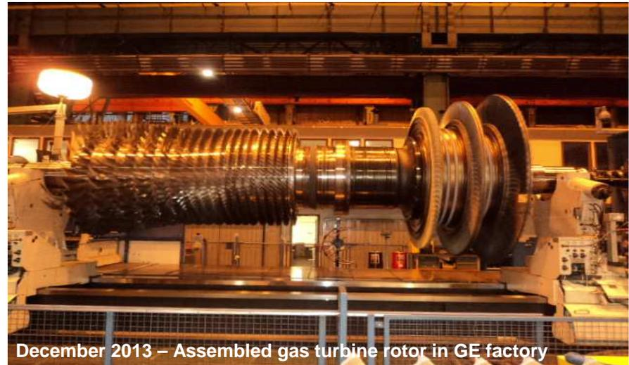
December 2013 – Assembled gas turbine rotor in GE factory
