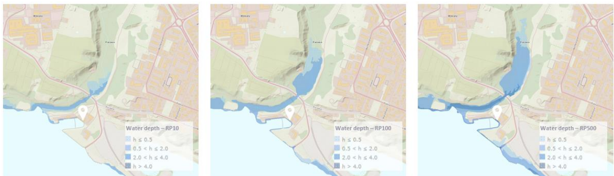
Figure 3-5: River flood hazard for RP10 (left), RP100 (middle) and RP500 (right) for the water intake facility (Wody Polskie, 2022).
